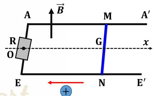
1. Determine the expression of the magnetic flux crosses the surface AMNE as a function of B, L, v and t, respecting the positive direction indicated on the figure.
